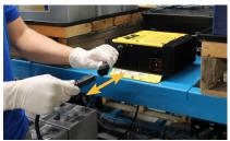
Figure 2: Disconnect AC power.
