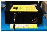
Figure 6: Red fault light blinking
