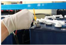
Figure 7: Touch the positive lead to the positive terminal for 3 seconds
